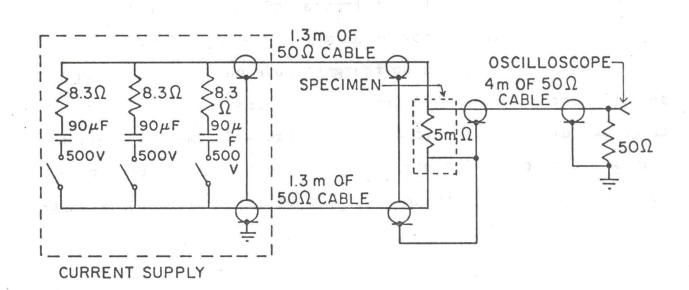
Fig. 3. Electronic measuring system.
